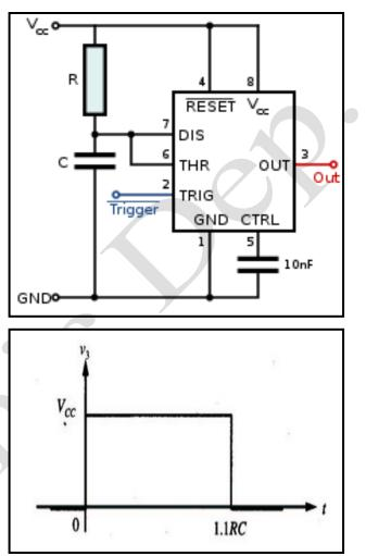
output to go low after a trigger pulse, the trigger signal muster turn to the high, VCC state. Otherwise the output will not reset to zero volts.
