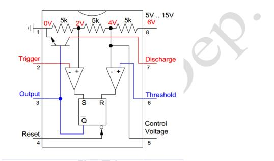
The functions of the pins are as follows (assuming a 6V power supply):
